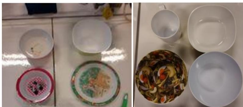
After the presumed migration, the melamine concentration in the different food simulants was measured with HPLC. To prepare the samples for HPLC, 1 ml of simulant together with 9 ml acetonitrile were mixed and evaporated. Finally the melamine was redissolved into 1 ml of the HPLC mobile phase and measured.
