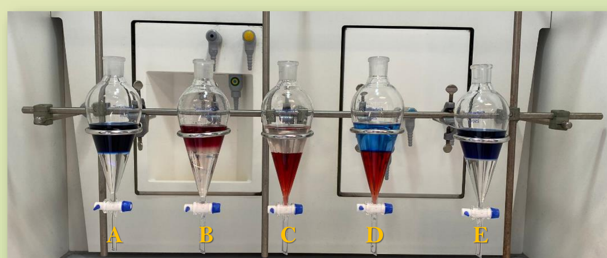
Figure 3: Colour change and phase transition as a function of change in pH and polarity
