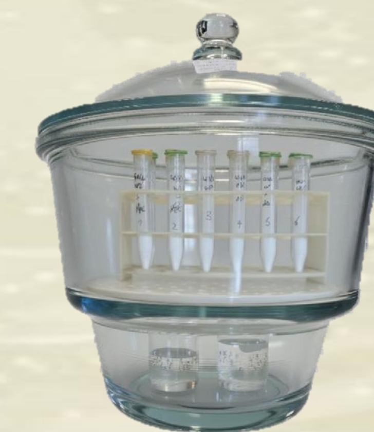
Figure 2: setups for water permeability testing of falcon tubes with bioplastic around the opening in a glass desiccator
