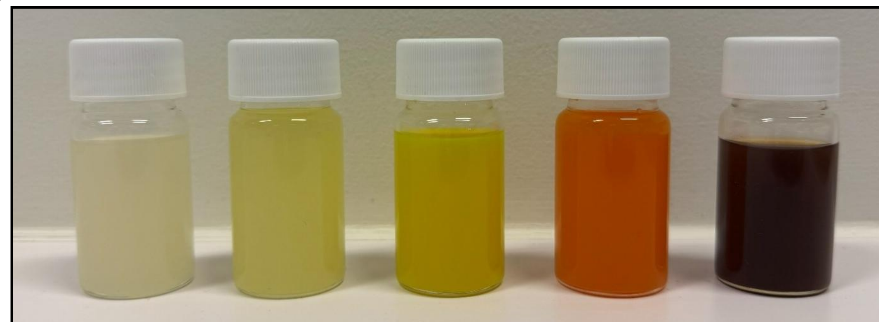
Figure 3. Fluorescence of CsPbX 3 perovskite quantum dots under normal light. Samples are arranged from left to right by halide composition: X = Cl, Cl/Br, Br, Br/I, I.
