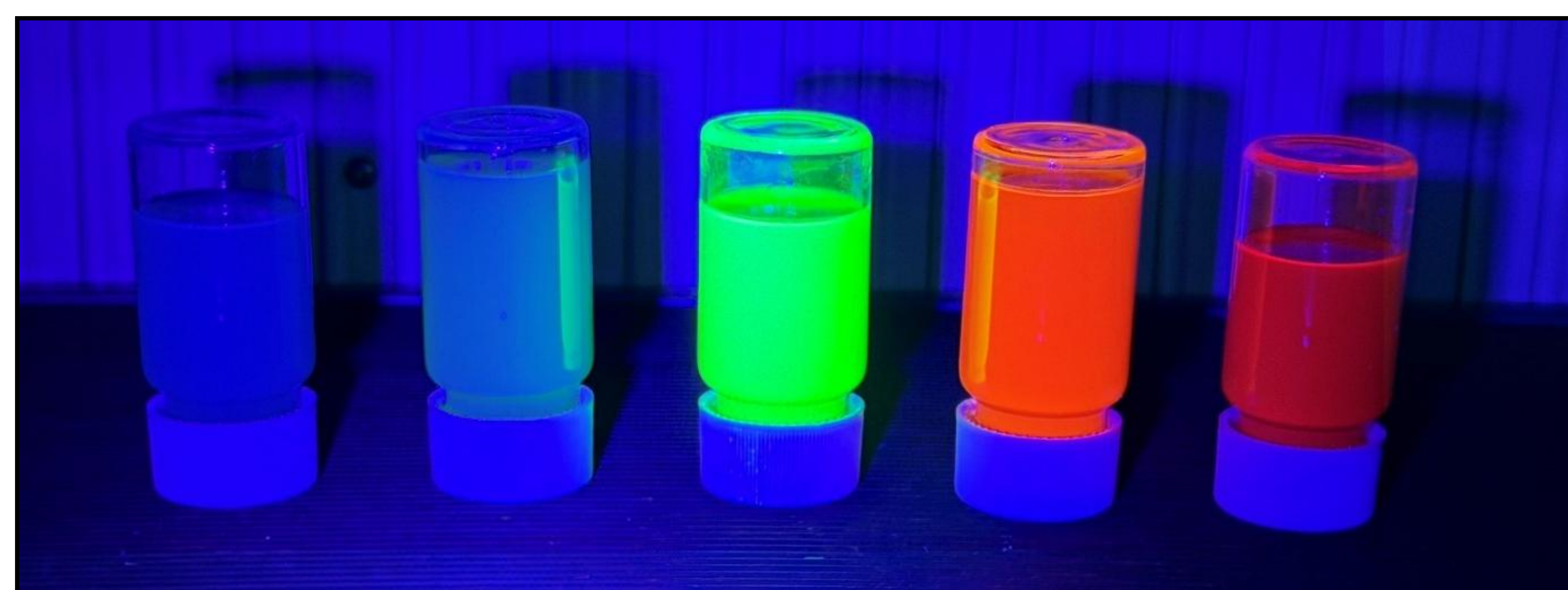
Figure 4. Fluorescence of CsPbX 3 perovskite quantum dots under UV light (λ = 366 nm) from a UV flashlight. Samples are arranged from left to right by halide composition: X = Cl, Cl/Br, Br, Br/I, I.
