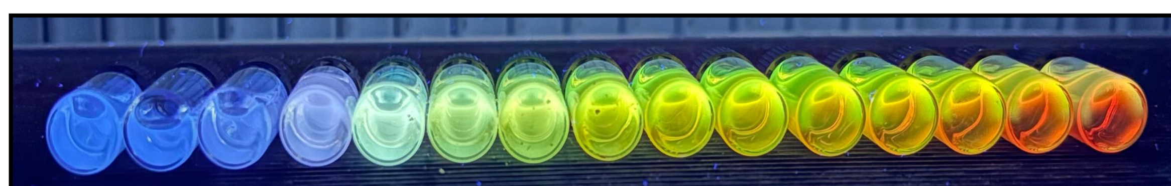
Figure 1. Fluorescence of CdSe QDs of varying size under 366 nm UV light.
